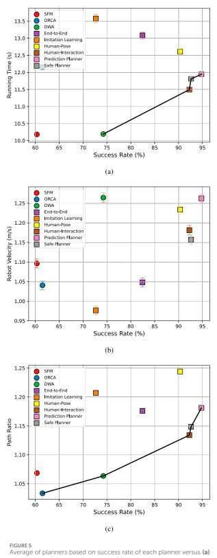
running time, (b) robot velocity, and (c) path ratio.
