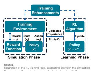
Phase, where the navigation model (policy) interacts with the simulation environment, and the Learning Phase, where collected experience is used to improve the model through the RL algorithm.
